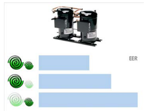
THE SEQUENTIAL DEACTIVATION OF THE COMPRESSORS INCREASES EFFICIENCY
